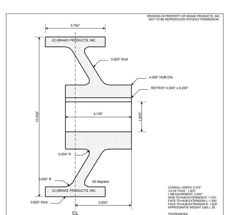
TOLERANCES: WHEEL DIAMETER: +0.005"/-0.000" BORE DIAMETER: +0.000"/-0.001"
